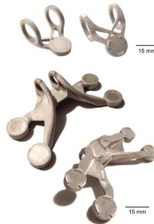
Fig. 2 Examples of parts made via ADAM in 17-4 PH [11]
