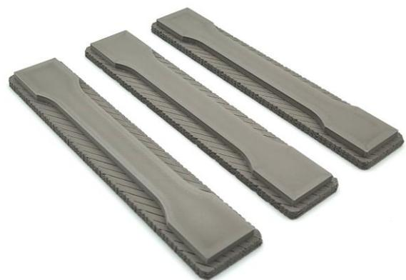
Fig. 3 Example of green parts printed via BMD in 17-4 PH stainless steel
