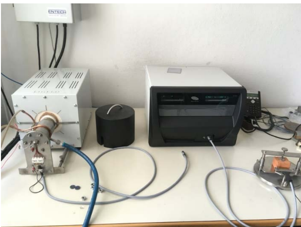
Fig. 2 Instrument Hot Disk TPS 2200
