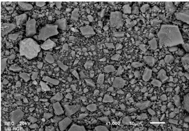
Fig. 1 SEM microphotography of basalt powder samples
