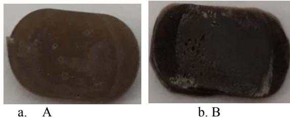
Fig. 2 Samples of A composite and B composite at the end of the testing time (60 min)
