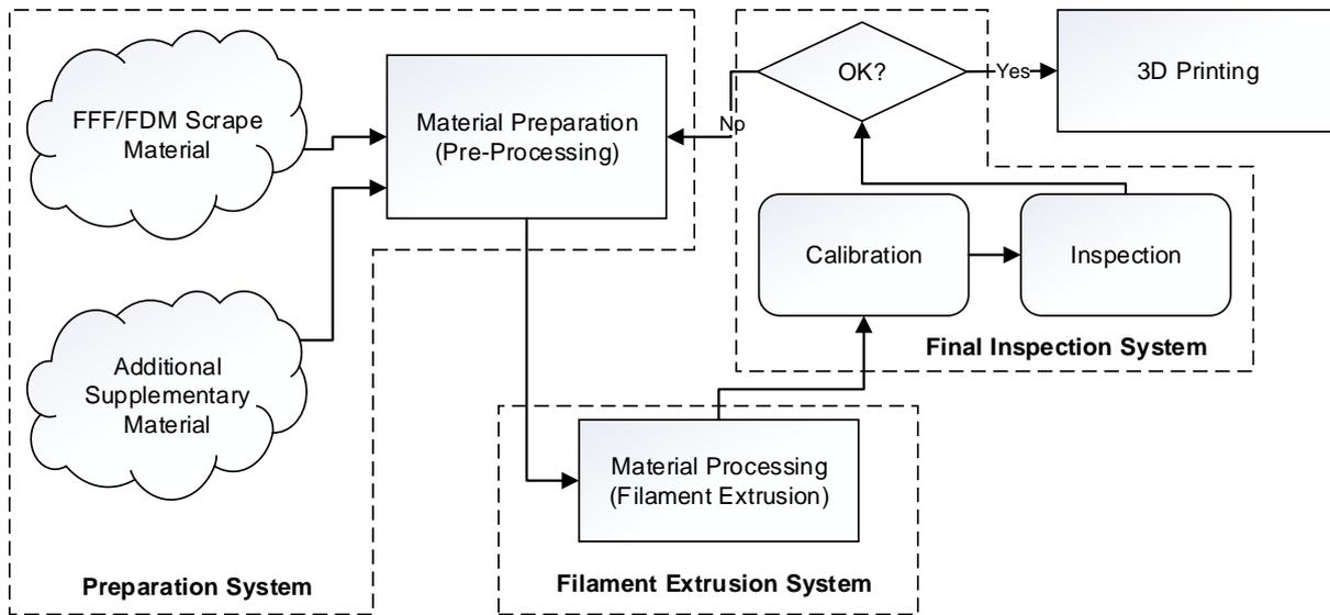
Fig 1. Schematic of the concept of FFF/FDM material recycling
